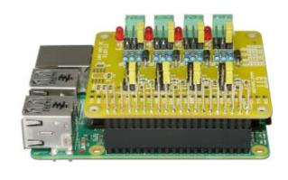
ET-OPTO DC-IN4 HAT is specifically designed for use with Connector 40PIN of Board RASPBERRY PI; this INPUT Board is 4-CH OPTO ISOLA-TION
