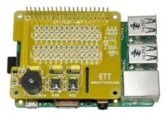
Board ET-TEST HAT is specifically designed to test I/O PORT of Board RASP-BERRY PI; it is used to test the operation or write sample program to show on LED Display or BUZZER on this board.
