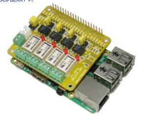
Board ET-OPTO RELAY4 HAT is specifically designed for use with Connector 40PIN of Board RASPBERRY PI; it is 4-RELAY Board.
