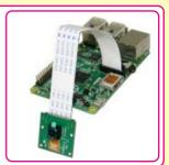
This MODULE CAMERA is specifically designed to use with Board Raspberry PI, it is compatible with MODEL A+, MODEL B, MODEL B+, Raspberry PI2 MOD B; moreover, it can be connected with SOCKET CAMERA as CSI BUS type
