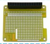
It illustrates how to connect ET-PROTO HAT, it solders 2 x 20 STACKABLE 25.5 mm. onto Board RASPBERY PI.
